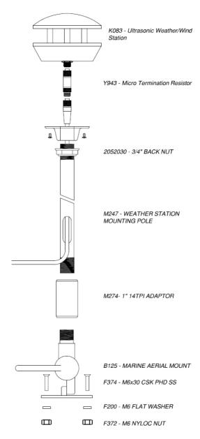
Figure 5-3. Outside Cab Weather Station Layout
